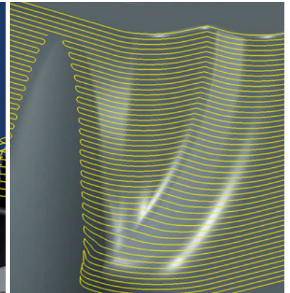
Zigzag machining of open milling areas
