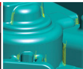
Machining of only steep areas
