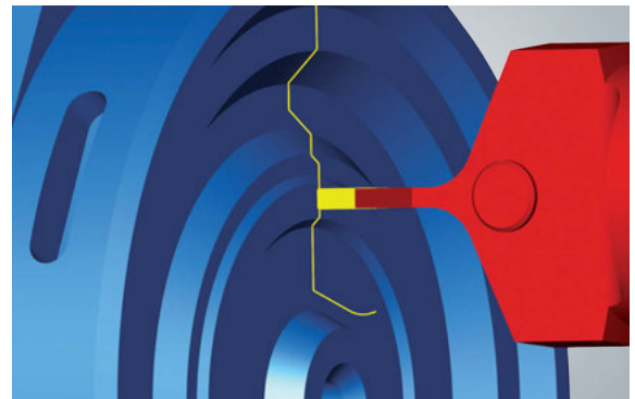
Face groove finishing: This strategy is used to finish axially aligned grooves and shoulders with a grooving tool.
